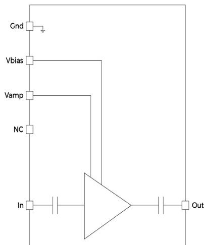
**Mechanical Diagram and Pinout**
