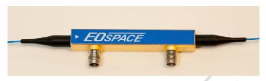
1550nm Ultra-Broadband X-cut Lithium Niobate Intensity Modulator with extended frequency operation to ~60GHz
